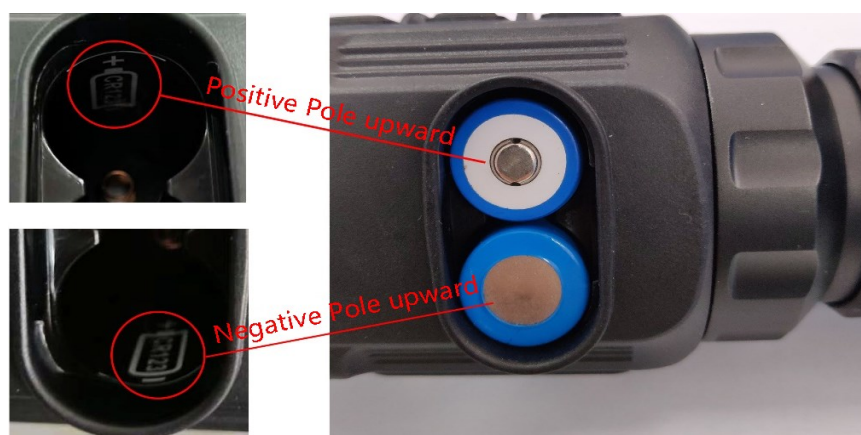
Fig.2 Battery installation
